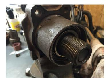
The below picture shows the threads on the large knurled nut and the undercut. The design of the tool ensures tool stops against the bearing face. It's important to have the undercut on this nut to reach the bearing.
