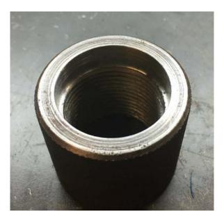
Install the large knurled nut (with the undercut side towards the bearing). Tighten by hand until all the slack is gone. The bearings will be seated in the races.
