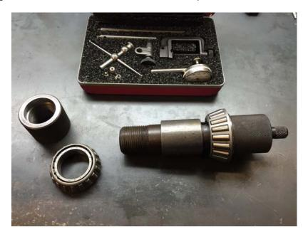
First, the inner bearing is placed onto the small end of the tool, pushed up against a stop on the tool and held in place by the small knurled nut
