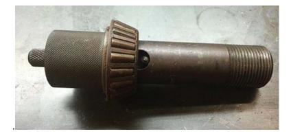
Tool is then placed inside the bearing housing, and the spacer slid on from other side. Spacer may be slid on before tool is inserted in housing.
