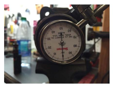
Move pin and read measurement. In this case, it was just over .039"
