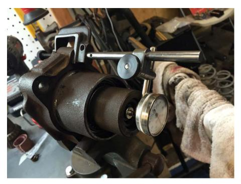
Push the center pin to one end of travel and zero out the dial indicator.
