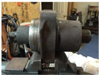
After tool, inner bearing and spacer is inside the housing, slide the outer bearing on.
