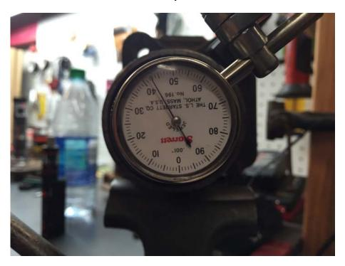
This measurement is then added to 0.097" for a value that equals the suggested shim size to be used. In this case, it came up with 0.136" to be used in this setup.
