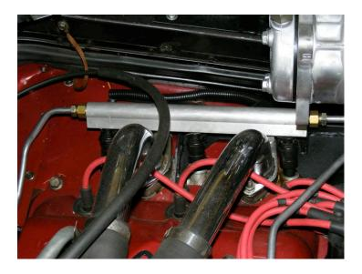
The only OEM fuel rail with Corvair's bore spacing was the big-block Chevy and those rails were hard to come by. Fortunately Accel sells blank fuel rail by the inch and injector bungs in sets of eight. The blank rails were drilled and tapped for injectors and supply lines. The fuel rails are secured to the cylinder head with small aluminum straps.
