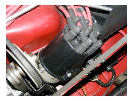
A mix of Corvair and Fiero, the lower portion of the Corvair shaft is mated to the upper section of the Fiero shaft. The bottom of the Fiero distributor bowl was machined smooth; it's screwed to an aluminum ring mounted in the Corvair's distributor bowl. The HEI ignition coil is mounted in the same place as a regular Corvair distributor.
