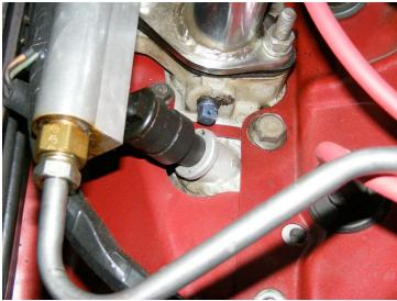
The machined bungs were heli-arc welded to the manifold. During welding, a fixture insured that the bungs were aligned with the intake valves.
