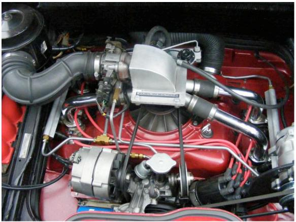
The plan was to adapt a complete system from a 6-cylinder donor which similar displacement and horsepower; this to minimize the cost and need for re-programming the ECM to match the engine. Why not take advantage of the millions of R&D dollars spent developing and testing these existing systems?
