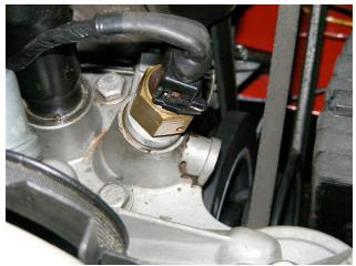
This sensor is mounted in the original fuel pump mounting hole where it senses oil temperature instead of the usual coolant. As the engine warms, there's less and less run-time for the cold start injector. When the engine is warmed up, there's no flow at the "cold-start" 7<sup>th</sup> injector.
