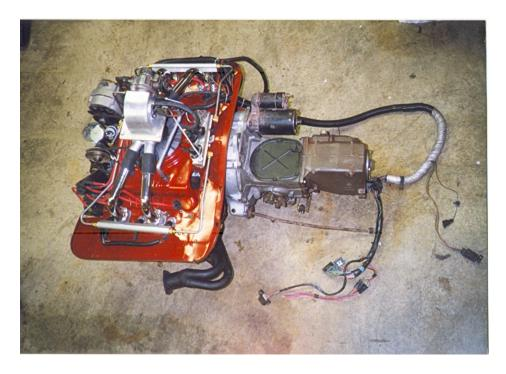
The stock V6 Fiero harness was widened to accommodate the Corvair flat six. Several quick disconnects were installed where the cable enters the engine compartment to facilitate engine removal, The Fiero harness included a hard grommet that protects the harness where it passes through the firewall, er, rear seat bulkhead:
