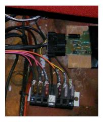
When the vehicle is stopped, the ECM uses the idle air motor to control the idle speed so the ECM uses a vehicle speed sensor to know when the vehicle is moving and when it's stopped. To install the VSS, the original speedometer cable was taken to a speedo shop where it was cut and fittings were installed to accept the inline vehicle speed sensor. The sensor output goes to a "VSS buffer" module that's next to the ECM.
