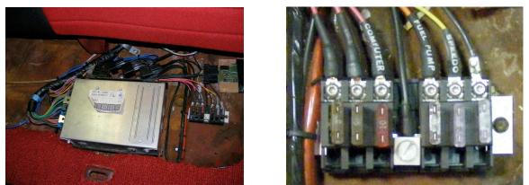
The stock Fiero ECM, with original 2.8 V6 programming, is located under the rear seat, as are relays for fuel pump & A/C compressor. The auxiliary fuse panel includes circuits for injectors, ECM, fuel pump, speedo buffer, and O2 sensor
