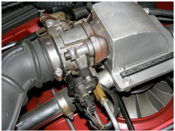
An aftermarket 140-4-bbl adaptor and fabricated air box distribute air from the throttle to the four cylinder head air intakes. The throttle flange from the Fiero intake is welded to the air box. To prevent throttle freezing, the original throttle included passages for circulating warm coolant, Instead of coolant, a turbo oil tee provides warm motor oil for the throttle while return oil dumps into the oil fill tube.
