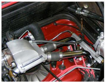
Originating from the bell-crank at the rear of the undercar tunnel, the long stock Fiero throttle cable is routed into the engine compartment where it connects to the Fiero throttle. Just for fun, the cable and grommet come through the shroud at a flat area designed for the automatic transmission dipstick.
