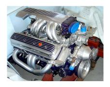
In 1985, Chevrolet introduced "Tuned-Port Injection" on the Corvette, and Camaro 305 and 350 Engines.
