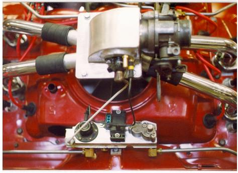
The Fiero's original V6 fuel rail, visible in the foreground of the photo, is mounted at the front of the engine using the original Corvair balance tube mounting points. Also on the original fuel rail; the fuel supply for the cold-start injector, fuel pressure regulator, MAP sensor, pressure stabilizer, and pressure test port. Four original injector holes were welded shut and two were tapped for fittings to the new rails.
