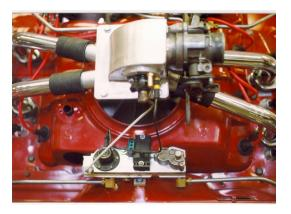
New steel hard-line runs from the in-tank pump to the fuel rails. Excess fuel in the rails is piped to the pressure regulator where it sends excess fuel back to the tank through the original fuel line. The pump mounting ring was grafted-in from an S-10 blazer tank. While the pump is capable of 90 PSI, the regulator spills most of the fuel back to the tank and maintains 35 to 45 PSI in the fuel system.
