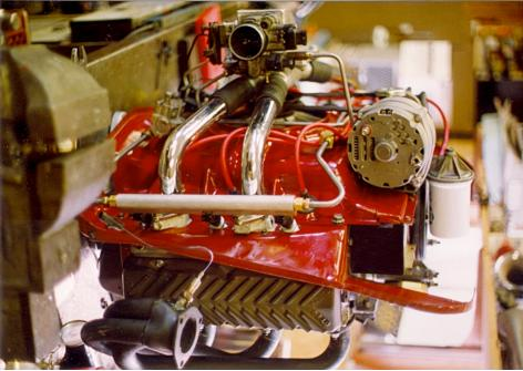
A heated oxygen sensor is installed in left exhaust header. This O2 sensor is rather distant from the cylinder head and early testing revealed that the original unheated sensor would cool off and stop working at idle speeds. Upgrading to a heated sensor cured the problem.
