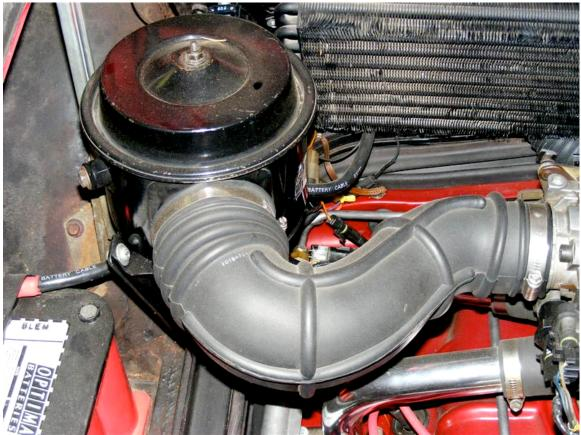
The stock Fiero air cleaner fit well but the Intake Air Temperature sensor was relocated to provide clearance for the deck lid support. Intake noise is effectively muffled by the thick rubber intake duct.
