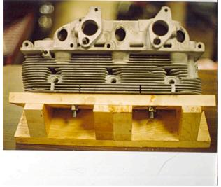
The underside of each bung was milled at a 45-degree angle so the inside of the intake manifold remained unobstructed.
